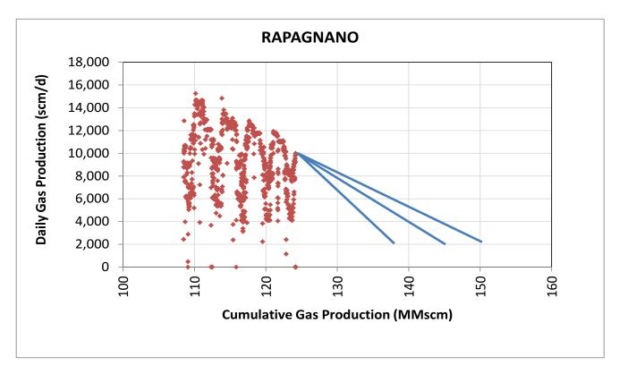
Figure 8-8 Rapagnano Gas Production vs Cumulative Gas
