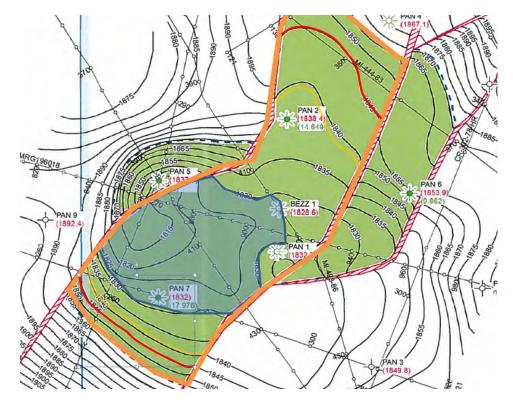
Figure 5-8 MI3-R Structure Map for Bezzecca-2 Volume Estimation
