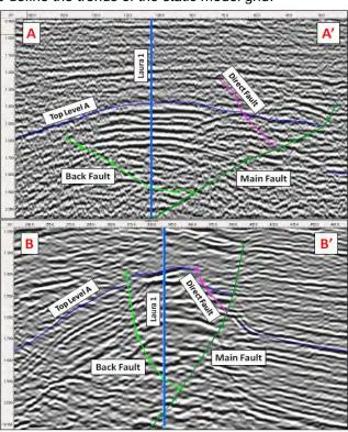
Figure 10-3 Interpreted faults (on the left) and seismic lines through Laura-1 well (on the right).
