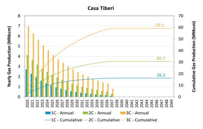
Figure 13-9 Technical Production Profiles of Casa Tiberi 1C, 2C and 3C (Sidetrack Well, before Economic Cut-off)
