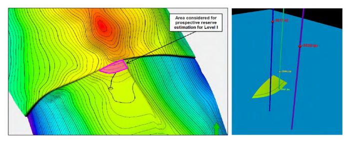
Figure 12-8 Boundary polygon (on the left) and related gross-rock-volume (on the right) used for Level-I GIIP estimate
