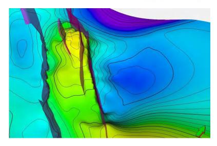
Figure 10-2 Structural map of the San Mauro Fm. Top and interpreted faults in Sound static reservoir model.
