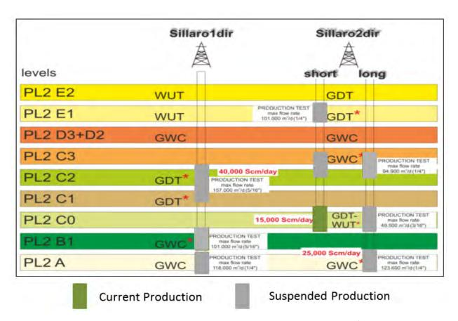
Figure 4-2 Sillaro Field Producing Levels and Well Completions (as of 31<sup>st</sup> October 2017)
