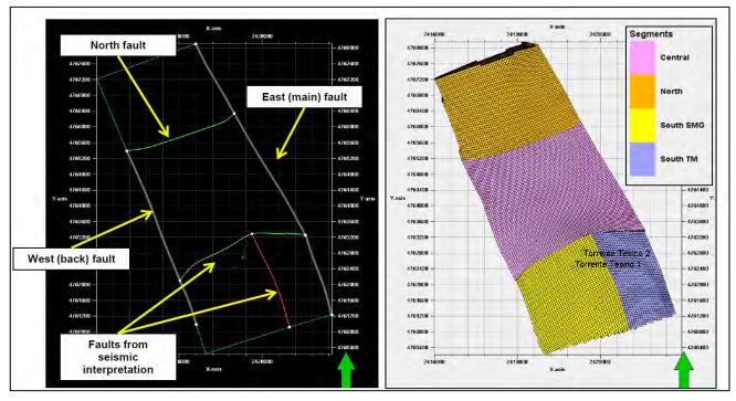
Figure 12-7 Grid and segments in the Apennine 3D static geo-model (source Apennine)
