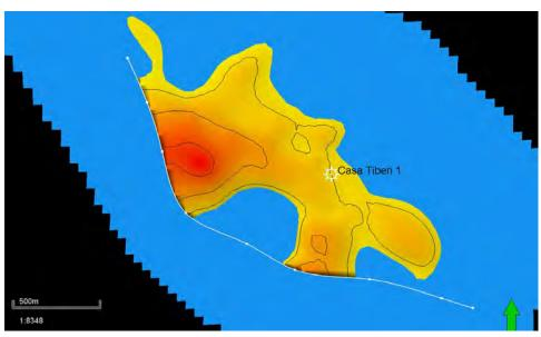
Figure 13-3 Location of Casa Tiberi-1 well, relative to Depth Structure and Aquifer at end 2017
