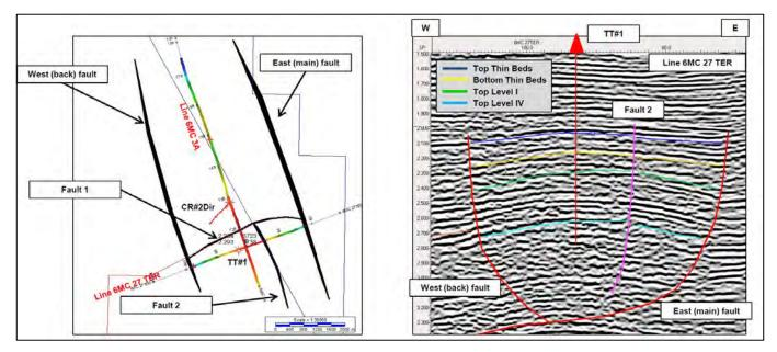
Figure 12-4 Schematic cross section (on the left) and seismic line (on the right) showing Fault-2
