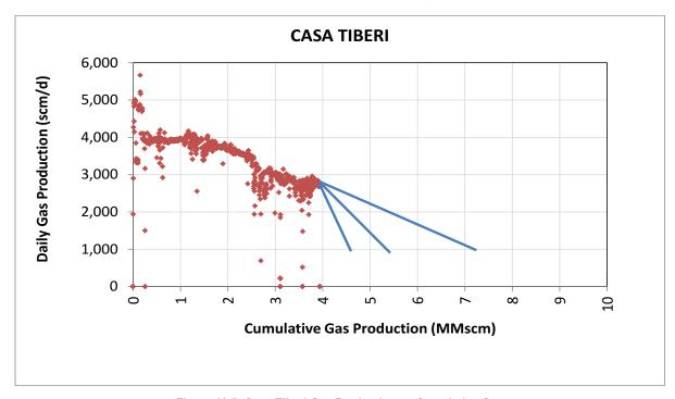
Figure 13-7 Casa Tiberi Gas Production vs Cumulative Gas
