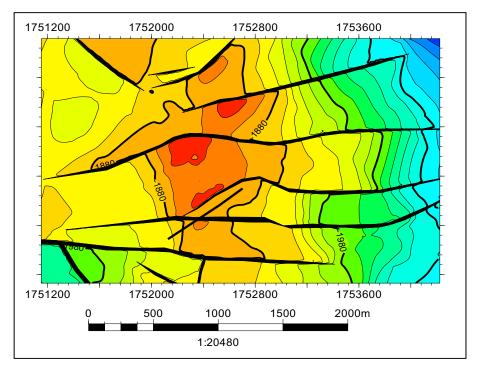
Figure 9-3 Depth Structure Map, 2017; Sant'Andrea-1 DirST Encounters small, fault-bounded compartment Source: Appenine Presentation (2017)
