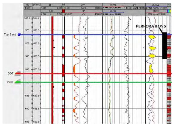
Figure 13-4 Casa Tiberi-1 Well Logs; Note Gas-Down-To (red line) and Water-Up-To (green line)
