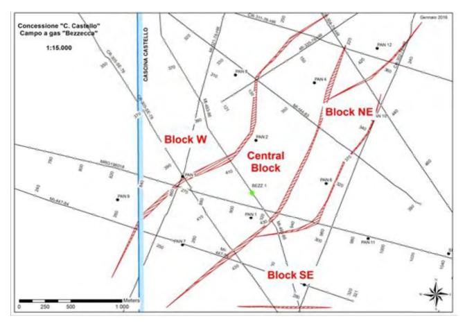
Figure 5-2 Identified Fault Blocks, Bezzecca Field
