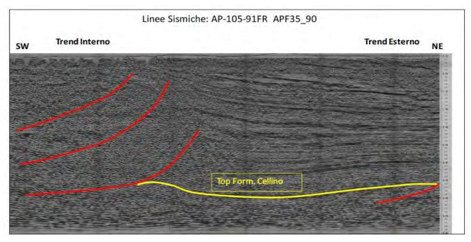
Figure 12-3 Seismic interpretation of the Internal (Western) and External (Eastern) trends (source Apennine)
